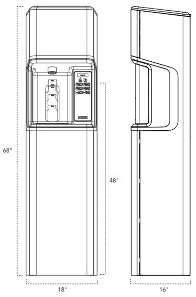
Note: If placing a Refill Station in an enclosed cabinet, please leave 3" clearance on each side, and 6" clearance to the rear. Ensure that there is sufficient venting.
